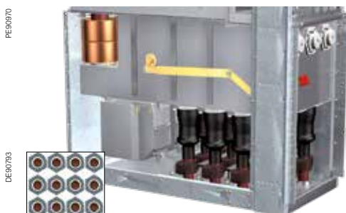
Inner cone-type bushings up to 40.5 kV, multiple cable connections (1x to 4x) size 2 (800 A) or size 3 (1250 A) with flange-mounted voltage transformers
