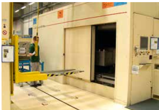
Integral routine leakage test
