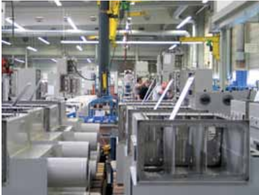
Completion of the WSA and WSB switchgear panels
