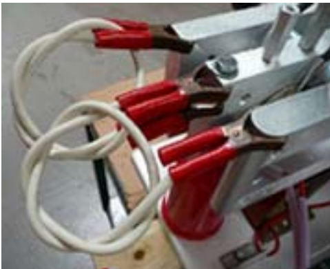
Figure 10: Ring transformer primaries to ground
