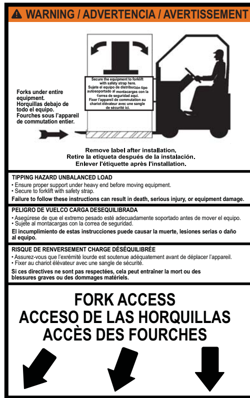
Figure 4 – Rear Warning Label, Rainproof Switchboards
