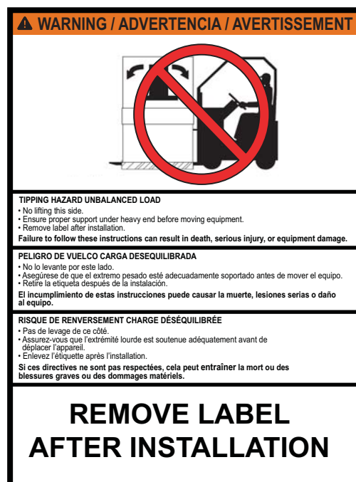
Figure 5 – Front Warning Label, Rainproof Switchboards
